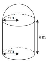
[A sphere of radius r has volume EMBED Equation.DSMT4  $\pi r^3$  and surface area  $4\pi r^2$ ]
